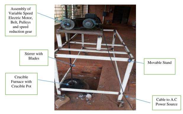
Plate 1: Fabricated and Improvised Stirrer Set up for Stir Casting
