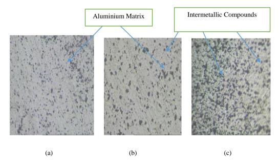
Plate 4: Optical Micrographs (100X) of Al/RHA Composites at (a) 6 wt.% RHA (b) 8 wt.% RHA (c) 10 wt.% RHA
